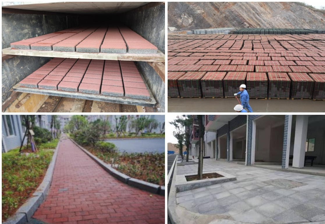
Figure 7. Non-sintered bricks and applications prepared from bauxite residue and other industrial solid wastes.
